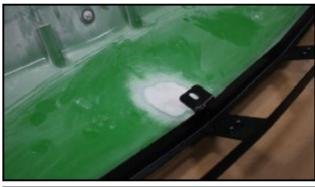
6. Remove tab. Use Sandpaper or a Scotch Bright Pad to ruff up the marked area until you remove all the paint. The epoxy needs to bond with the fiberglass, not paint. Clean the surface of all dust once completed.
