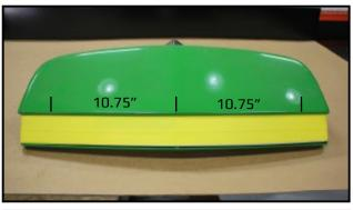
1. Remove front nose from hood, may have to cut decals. Find Centerline of front nose, after finding center-line, measure 10-3/4 inches both ways of centerline. Before you cut, give yourself about 1/8" of clearance. You will want to file to fit to 10-7/8. 10-7/8" is **MAXIMUM** from centerline.
