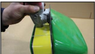
Next cut on the bottom side of marked line. You will want to file to fit as well.
