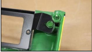
5. To install the Tab, bolt the light housing into the nose. Then, bolt the tab into the housing. Align the tab square with the housing, and make marks onto the nose outlining the tab.
