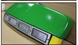
9. Install lights into light housing and secure with bezels and screws. Take care to install lights all the same way for wiring making sure the wiring tabs are all facing the same way. Wiring should be on the right side of tractor. Lights are polarity specific, RED to +, black to -
