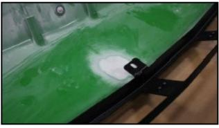
6. Remove tab. Use Sandpaper or a Scotch Bright Pad to ruff up the marked area until you remove all the paint. The epoxy needs to bond with the fiberglass, not paint. Clean the surface of all dust once completed.
