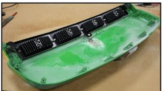
8. After 10-15 minutes remove 3 bolts to remove light housing. Paint if desired. After painting, reinstall nose to hood without light housing. Once nose is installed on hood reinstall light housing.
