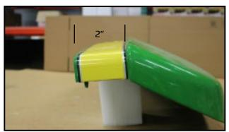
2. Measure from bottom of nose to where we will cut. The measurement should be 2"
