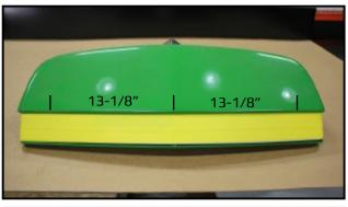
1. Remove front nose from hood, may have to cut decals. Find Centerline of front nose, after finding center-line, measure 13 inches both ways of centerline. Before you cut, give yourself about 1/8" of clearance. You will want to file to fit to 13-1/8. 13-1/8" is **MAXIMUM** from centerline.
