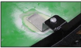
7. Apply a thin layer of epoxy between tab and nose. Install tab and place remaining composite on top of tab. You will need plenty to cover tab and about 1/2"-3/4" around tab. Let sit for 10 -15 mins.
